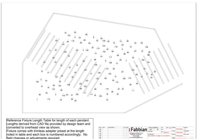
The installation was simplified by having the trimless adapters set to the desired lengths for each of the 140 locations. Then each pendant was mapped to a specific location, and pendant boxes were clearly labeled with locations. Once the trimless elements were mudded into the ceiling, a simple 24V plus and minus connection at each location was needed to finish the installation. Revit files were integral to this process.
